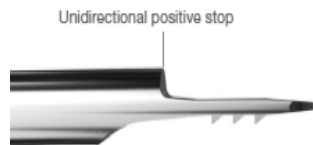
Figure 2: Positive Stop Feature, Access Chisel
